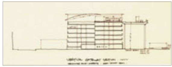
This sketch illustrates how new buildings and structures (including parking garages) can provide a link between the street system on the Valley floor and the historic bridges that cross the Valley.
